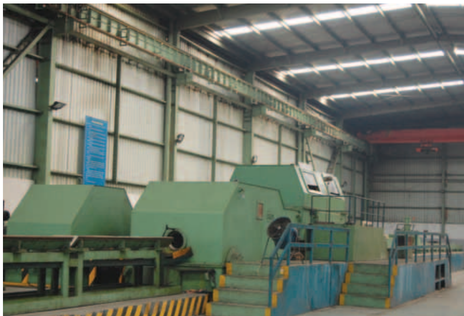
Model 280 Cold-rolling Line can handle pipes with an O.D. up to 325mm
