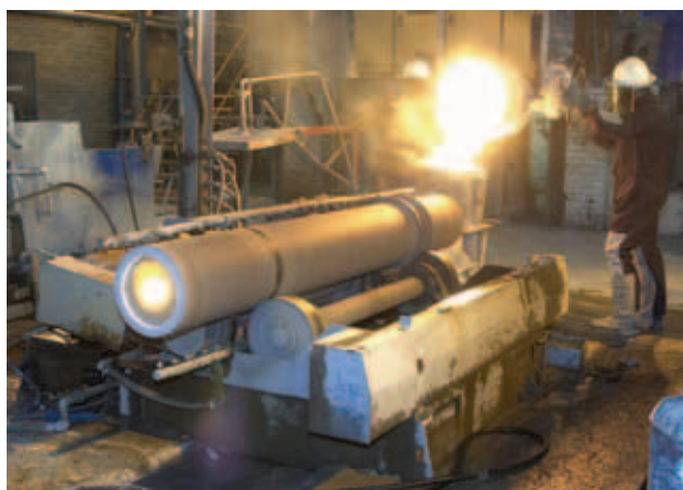
Steloy Castings is one of a handful of foundries in the world able to cast process tubes in high-alloy steels.
