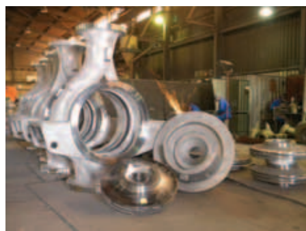
Recent contracts, clockwise from top left: Steloy cast 400 x 42” stainless steel cryogenic valve bodies and discs for Middle East oil and gas; supplied 196 sets of reformer tube components to a Hawaiian refinery within four weeks; is supplying chrome steel pump components for two SA coal-fired power stations, and cast 30 X 1,230 kg diffuser bowls in super duplex stainless steel for a Middle East desalination plant.
