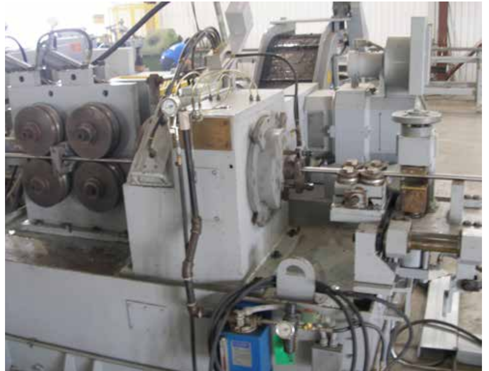
A hot rolled bar enters the Hetran bar turner, while a peeled bar exits.
