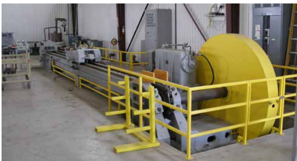
A 23-foot (7 m) draw bench for high reduction.
