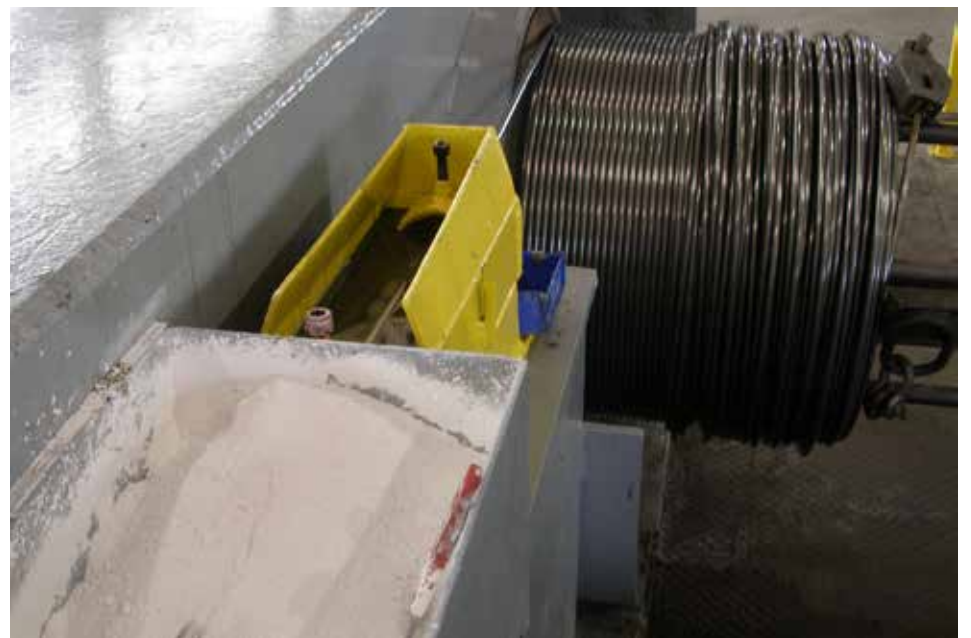
A horizontal 'bull block' cold drawing (coil-to-coil) process (close-up in inset).
