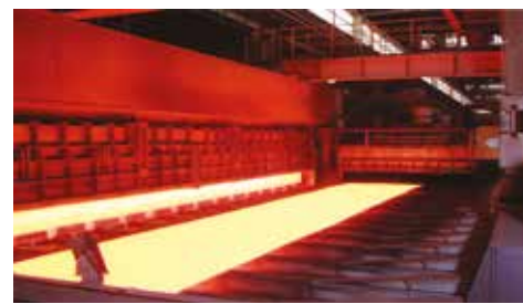
The annealing process at the Kawasaki Plant.
