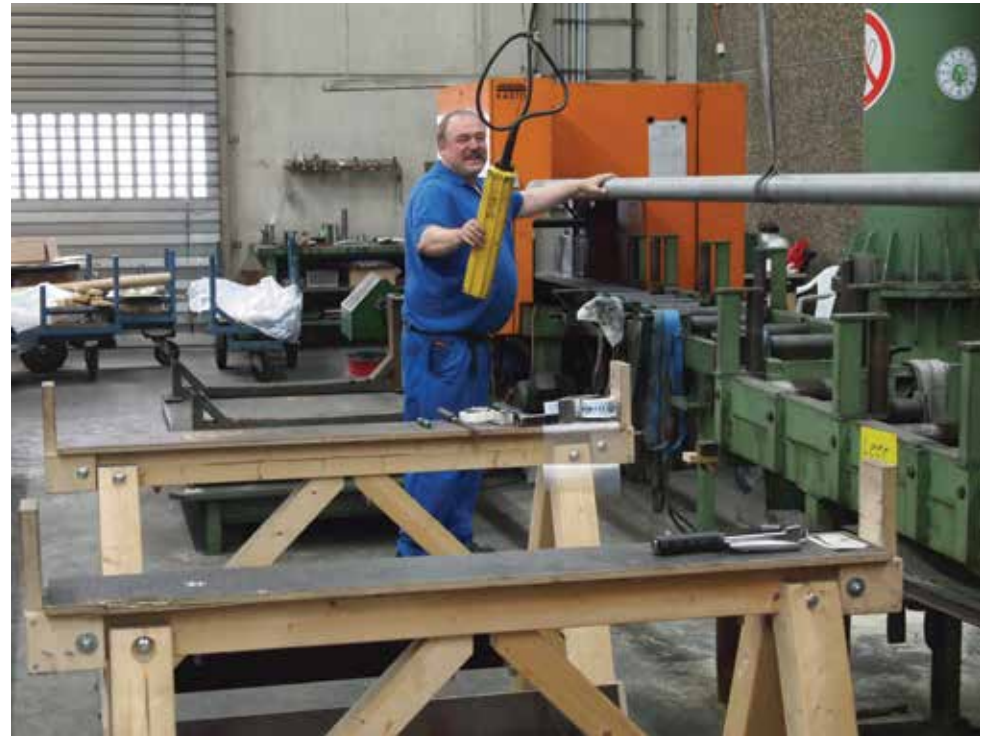
Machining according to customer requirements: in the sawing machine, the tube receives the desired length.
