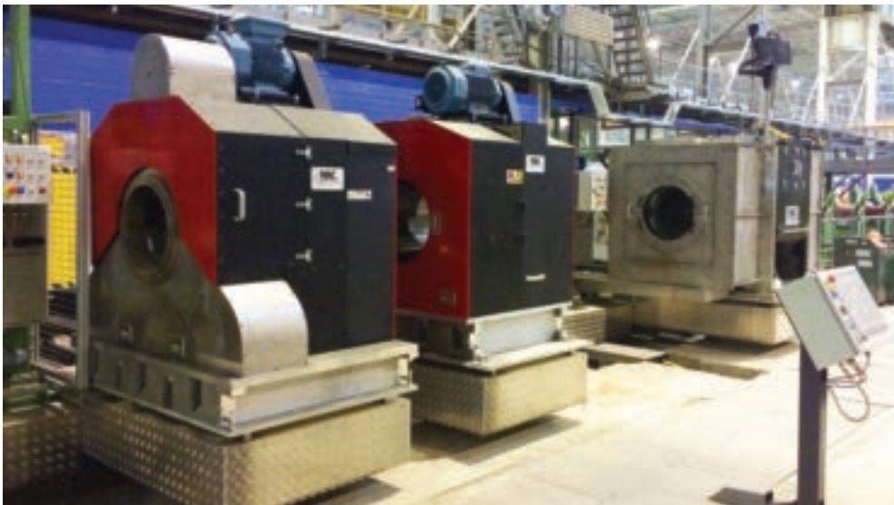
A complex test system designed to meet API standards for OCTG pipe at a Russian mill. Included is MAC's Echomac® 500mm Ultrasonic Rotary, at right, and Rotoflux® 500mm Transverse and Longitudinal Units at left.
