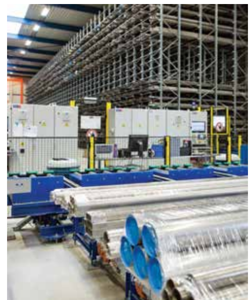
The new fully automatic Fehr Honeycomb storage system.
