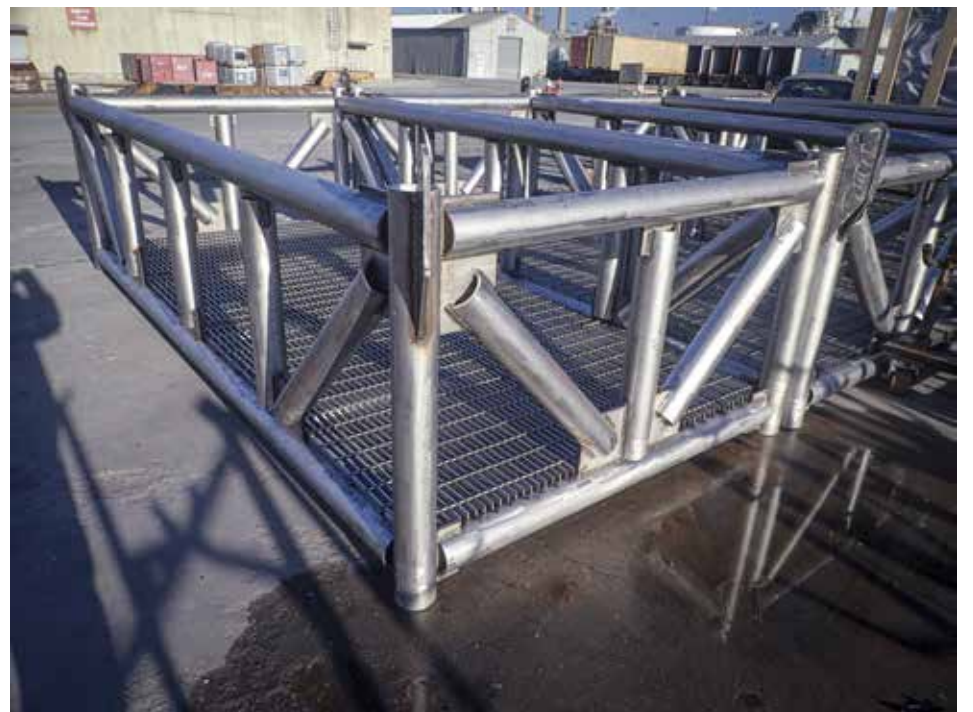
The finished furnace baskets made of 304H pipe provided by MRC Global to Ascend Materials.
